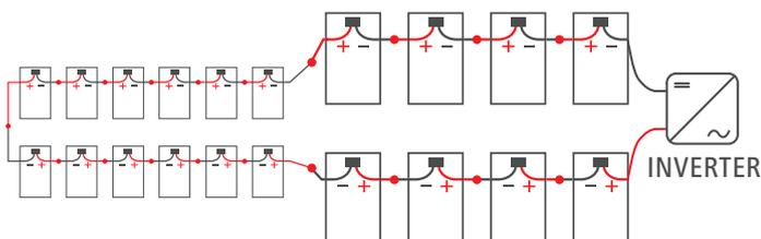
● DC plug connection (connection points between male and female connectors)
